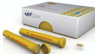
Water can occur in jet fuel in three forms, dissolved (chemically in solution in the jet fuel), settled (as in free water at the bottom of the tank), or as finely dispersed undissolved water held in suspension. The Shell Water Detector is designed to detect undissolved water; it has been proven reliably for 30 years. This is water
