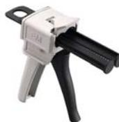
This Plunger is for the Scotch-Weld™ EPX™ Plus II Applicator. The Scotch-Weld™ EPX™ Plus II Applicator is used to Dispense 3M™ Scotch-Weld™ Adhesives in Duo-Pak Cartridges. The applicator is a low-cost portable, self contained metering, mixing and dispensing machine that simultaneously meters and mixes two-part adhesives as the material is applied.
