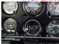
Designed with static cling polyester, the IIA will stick to your glass instrument face without licking and will stay there until you want to remove it. Practicing instrument failures during flight is a requirement by the Federal Aviation Administration for your practical test. One package includes four Inoperative Instrument Aids. Developed by a Certified Instrument Flight Instructor with the intent to
