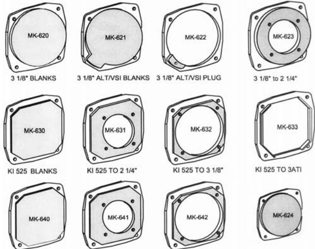
CNC Machined from aircraft grade aluminum. The adapter face is raised .075" to give the flush panel look. Easy to install and easily painted.
