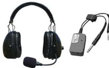
The EQ-Link Headset offers wireless freedom in the aviation cockpit. The EQ-Link module plugs into standard general aviation inputs on the aircraft's audio panel and provides a 2.4 GHz frequency hopping link (not Bluetooth®) to the EQ-1 ANR Headset. Now you can enjoy all of the features of a premium ANR headset with none of the wires!
