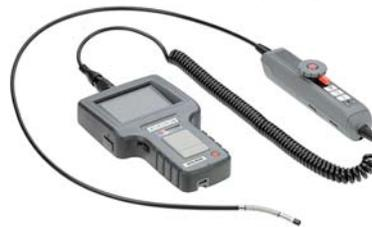
The state-of-the-art ATS Voyager videoscope features an articulating tip that swings 240 degrees to reach every inspection point of an airplane. With a simple turn of the control knob, you can move its Tungsten-sheathed tip from side to side to look left, right, and even backwards! The ATS
