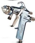
The Binks Mach 1 HVLP is a siphon-fed refinishing system that performs like your favorite conventional outfit but produces far superior transfer efficiency. A unique arrangement of air nozzle, fluid nozzle, and needle enable the Mach 1 to draw material from a standard siphon feed cup and avoid the need for a pressure cup. Eliminates the need for the operator to set fluid pressures. Delivers lower emissions for
