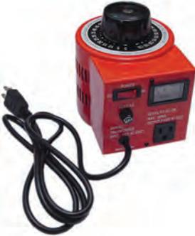
A fine quality control to supply the electrical current for hot-wire cutting of styrofoam and PVC foam. One unit can serve to build many aircraft. Input 115 volts AC Output variable from 0 to 130 volts AC at 5 amps Caution - fuse should be inserted in the secondary to protect the control in the event of a short circuit.
