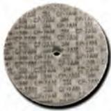
**Two Styles Available:** Cut & Polish/Unitized Wheel-7A Medium grade (harder) Use to radius and deburr edges of aluminum parts. These wheels give a uniform brushed satin finish to parts and deburr quicker and easier than hand finishing. These wheels are discs of Scotch-Brite web compressed and bonded to form a rugged, dense wheel. Wheel size: 6" dia. x 1" wide x 1/2" thru hole.
