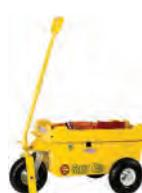
**MODEL 3324** - Combination power supply and battery pack. Batteries: \* 78 Amp Hours at 10 hour rate \* 24 Volt DC - 25.5 Volts at rest Sealed cells non-hazardous Valve regulated high amperage output lead acid \* 3200 Peak Amps Power supply / charger: \* Multi-unit 58 Amp DC continuous output \* 28 - 28.5 Volt output from 0 - 58 amp load \* Battery recharge time from fully discharged - 2 hours \* AC Input - 110 Volt or 220 Volts (only 1) Limitations : 200 amps maximum DC load.
