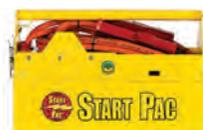
**MODEL 2300 QC** - Built in chargers, power plug and cables. 24/26 VDC output, with universal chargers that will accept 90-240 VAC 50/60 hertz. \* 26 AMP hours @ 10 Hour Rate \* 2300 AMPS Peak Current \* Trolley avail. \* 19.2"x7.5"x11.5" \* 69 LBS. Complete. For starting engines up to 1500 horse power and give four to six starts between charges. This unit has a dual redundant
