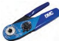
The Daniels AFM8 is designed for most of the miniature and sub-miniature connector types that are so widely used in all types of electronic systems. Originally developed for the Air Force, the AFM8 meets the need for a miniature tool accommodating wire sizes 20 thru 32 AWG. The cycle controlled precision ratchet assures consistently accurate crimps every time. The tool has a built-in eight step selector knob for ease in dialing the correct crimp depth setting for the wire being used.
