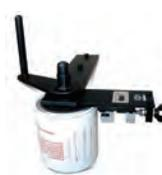
This tool was designed to eliminate much of the mess that occurs with small handheld oil filter cutting tools. Very simple to operate, it is excellent for individual aircraft owners as well as FBO's and maintenance shops where a lot of filters need to be cut. Simply clamp in a vise, screw on the filter, turn the cutter into the filter and hand crank to open the filter. The rugged construction enables this tool to operate trouble free for years.
