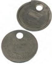
This gap gauge provides easy accurate spark plug adjustment. Features flanged edge for electrode bending and beveled round hole for opening gap. 1-1/2" diameter. Wt.: 0.8 oz. Scaled from .020" to .100". Pewter plating makes the inches more legible for user to read. Also available in metric scale (0.5 mm to 2.4 mm). Gap gauge (inches)
