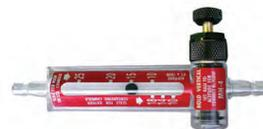
The MH-4 has two altitude flow scales. The left (compressed) scale is calibrated for the Oxymizer™ cannula and is limited to flight of 18,000 ft. and below. The right scale is calibrated for a standard cannula or facemask up to 25,000 ft.
