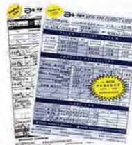
Simplify VFR or IFR navigation with these handy logs which provide for listing of intersections, radials, frequencies, clearances and complete flight plan.
