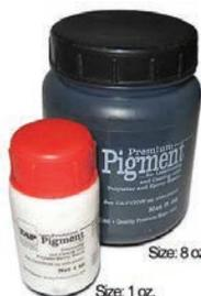
These Premium Pigments are a paste to tint polyester, vinyl ester, epoxy resin, and polyurethane. Add about 6% to 8% of pigment by weight or 1/2 pint of pigment per gal. of resin.
