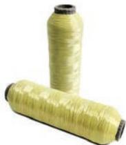
Material: 1500 denier Twaron (aramid), 5 ends (7500 denier total). Type: 1000. Yield: 567 yards/pound (0.588 lbs/1000ft). Elongation: 3.5%\* (each end). Break: 79 lb. +- 6.25%\* (each end) Packaging. Tube length: 5.25". Inner diameter: 5/8". Yards/package: 300 300 Ft. Roll.....P/N 968.....
