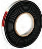
This is a 1/8" thick by 2" wide self adhesive tape that can be placed on metal panels and wrapped around ducts to reduce vibration and reverberant noise transfer. Not FAA approved. 30 ft. rolls.
