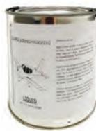
A paint-on soundproofing material that is applied to metal surfaces to reduce vibration and reverberant noise. Use to fill cracks and spaces where noise can enter. Buff color and can be painted. Paint engine mounts to increase fire resistance! Odorless and non-toxic when dry. Waterbased product. Non-Flammable. Shelf life: 1-year. Not FAA approved.
