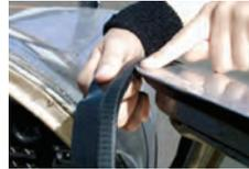
The "Spring-Steel" reinforcement channel has "Gripper" teeth to hold firmly in place. And when your door is closed the seal is pinched between the airframe. You can not pull the seal out when the door is closed... however applying adhesive into the channel is recommended. Length: 9ft.
