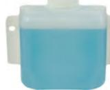
Constructed of high density polyethylene, this blow molded multi-purpose tank offers excellent durability and resistance to most chemical and fluids. All sizes nominal. Height includes neck & fittings. Width includes mounting tabs. Max working temperature is 180-deg F and max working pressure is 5 PSI. Capacity: 1.5 qt. • 7.74" L x 3.62" W x 5.9" Hgt.
