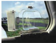
Very popular with Piper owners who need quick, high volume ventilation during ground operations on hot days. Kool Scoop is very easy to mount; simply peel off the adhesive backing sealer and stick it in place on the side window. It will fit any side window vent that does not have a thick frame. Made of top quality plexiglass. Really "scoops" the air from the outside to keep the pilot and passengers comfortable. Window frame not included.
