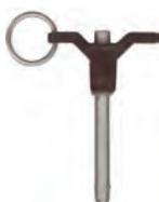
These pins of stainless steel, are made to exacting standards. Pushing the button on top, it contracts and releases two (or four) balls at the end of the shank. These balls lock onto and release from the part for fast removal. The following types and sizes are most commonly used for hang gliders and not for structural aircraft. Request quote on special sizes (25 piece minimum). Less 10% for 12, Less 15% for 25, Less 20% for 50. May be assorted.
