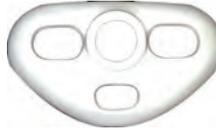
This design can be used with most any Continental or Lycoming engine. Used on the original Smith Miniplane but has been installed on the Pitts, EAA Biplane, Playboy, Flybaby & Baby Great Lakes. Measures 35" wide by 19.5" high. Face of center opening 8-1/2" O.D. P/N 05-01182 .....\$129.85
