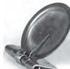
These 1" diameter spring loaded access doors can be riveted into your wheel pants. They open inward, so that using an appropriate tool, you can check pressure or inflate your tires easily without removing the wheel pants. Made of stainless steel which can be polished if desired. ....P/N 05-02124 .....\$39.85 ea.
