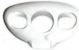
Identical to the MC-3B, but, has an opening for an oil cooler. Measures 35" wide by 21" high..P/N 05-01186 .....\$151.75
