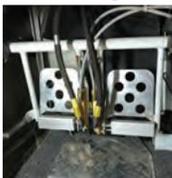
These very high-quality parts add considerable structure, feel and comfort to the Vans Rudder pedals. Pedals are cut from very strong and tough, type 6061 T-6 high tensile aircraft grade aluminum extrusion, with a very durable clear anodized finish. Pedals measure 4.5" X 1.5" X .75", are very light, 5 oz. each, feature simple and easy installation with only one bolt, and are very inexpensive as well.
