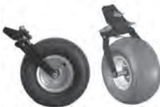
The T-11D tail wheel utilizes a dual fork configuration and incorporates a geometric release mechanism that allows the wheel to caster after reaching a steered angle of 40 degrees. The MH5N-S wheel used on the WHLT-11D has a .625 precision sealed ball bearing which is rigorously tested and designed to resist bearing fatigue providing a long bearing life.
