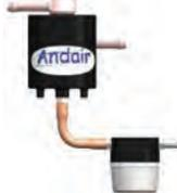
The OS8850 has been designed to remove the oil from the crankcase breather on Lycoming and Continental Engines. This gives reduced oil consumption, cleaner aircraft, and environment. \* Upper outlet can rotate through 360° allowing easy installation. \* The unit can be dismantled for inspection/cleaning. \* Vortex swirl separation. O-Ring seals. \* Light weight: 6.4 oz. \* 4 off 10-32 mounting lugs on the base of the separator for easy fire wall mounting.
