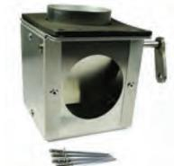
P/N DL-015 - This box is identical to the standard cabin heat box, P/N DL-001, except that the air intake is parallel to the firewall rather than coming straight in from the heat muff. This gives the builder the option of running scat tube parallel to the firewall. Total weight is 5.2 ounces and has a 2" inlet/outlet port. Furnished with a flange gasket and four mounting rivets. Can also be bolted to firewall.
