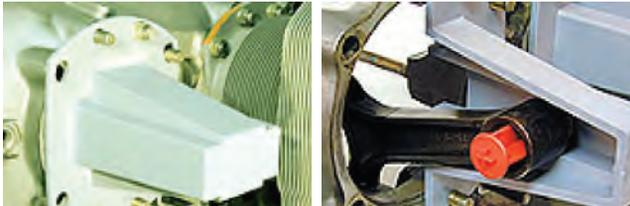
Install TopCap in place of a removed cylinder to protect the engine from dirt, debris, and stray parts. Made from fuel and solvent resistant polymer, TopCap allows for full crankshaft rotation. One size fits Lycoming wide deck 320, 360, 540, 720 and Continental 470, 520, and 550....P/N 08-00373 ... **\$24.75 /pr.**
