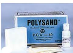
This is the original Poly-Sand process. Consists of a series of cloth-backed cushioned abrasives which when used in proper sequence will restore the finish of plastics. Also used for fine finishing of wood and precious metals. Recommended by Rohm & Haas Co., manufacturers of Plexiglas. Kit includes series of Poly-Sand cushioned abrasive cloth tapes, all required accessories and instructions.
