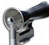
This venturi develops 4" Hg suction from double-throat venturi and 10" long horn. Used to operate a directional gyro or gyro horizon. When operating a directional gyro there is sufficient capacity to also operate a turn/bank. All aluminum construction. May require a suction regulator. Wt. 0.9 lb. ....P/N 15050 .....**\$89.75**
