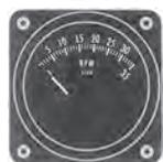
This tachometer is driven with power supplied by a transducer on the engine tach drive. Range 0-3500 RPM. Wt. 6 oz. Includes Gauge, sender, and tang.
