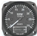
3 1/8" Analog Tachometer with hourmeter. 4 Cylinder. 0-3500 RPM. Records engine time above a set RPM point. Standard set point is 1800 RPM. Engine Type: Continental/Lycoming. TSO'd Magnetic pickup for Slick or Bendix Magnetos (6 ft. cable length), alternative to p-lead connections.
