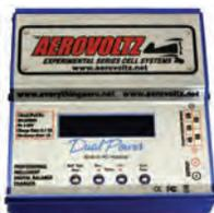
The only charger on the market designed specifically to work with the Aerovoltz battery. The primary advantage is the balance charging function. The Balance mode balances the voltage of each cell or cell pack while charging. By balance charging your you insure that the battery is operating at its maximum power. Periodic balance charging can also double the expected life of your battery. This charger is not required to operate your Battery, but it is highly recommended.
