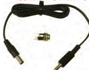
Auxiliary Charging Port for the Quiet Power Chargers. Auxiliary Charging Port Kit comes complete with a device specific charging cord and a barrel power jack (2.5mm ID x 5.5mm OD). The barrel power jack is designed to be panel mounted, allowing for quick disconnect of the charging cord.
