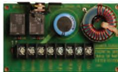
The Power Guard Module manages up to 10 Amps of secondary power for aircraft accessories that require back-up power. Typical accessories include electronic ignition, electronic engine/flight instrumentation and EFIS systems. The module works with a small 7-10 A secondary battery. The on board circuitry includes a secondary battery master relay, primary power controls, filter and charging circuit. **Dims:** 4.75"L x 2.75"W x 1.2"H ..... P/N 11-02044 ..... **\$169.99**
