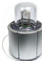
This precision compact unit mounts easily on top or below fuselage, and directly replaces rotating beacons. It features a high-intensity Xenon arc lamp, a high-efficiency push pull inverter circuit for stable flash voltage and a flame-resistant military circuit board assembly. The lamp is readily replaceable without removing the unit from the aircraft, and the unit weighs only 1 lb. 4 oz. The Flight Strobe FS-4400 is visible for over 50 miles at night, in haze, smog or bright sunlight and is
