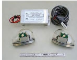
This new wing tip, 100% LED, strobe and navigation light system features a cluster of very bright LEDs and using a common controller that furnishes the heads with a junction point for synchronizing and selecting one of the 7 flash patterns of the LED STROBES. It also allows for a separate power source to the navigation red, green and white LEDs.
