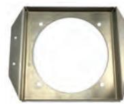
This flush mount bracket is a neat solution to mount a Garmin G5 standby EFIS to your panel. This aluminum mounting bracket can be fixed vertically or horizontally depending on your needs. There are 4 holes for #3 rivets to fix the mounting bracket to the panel. See Garmin G5 Flush Single for panel cut-out dimensions. Can be rotated 90 degrees if needed for panel obstruction. ....P/N 11-15457 .....\$59.75
