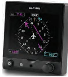
Glass Upgrade for DG/HSI and Attitude Instruments in GA Aircraft
