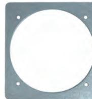
The G5 adapter plate is fabricated from 0.050 thick 2024-T3 aluminum per the dimensions shown in Figure 4-11. Apply a finish coat of paint to adaptor plates as desired prior to final installation. These may be field fabricated if needed and must have some type of corrosion protection (primer, alodine, etc.).
