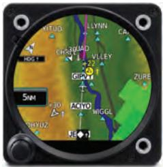
The GI 275 Base variant can be utilized as a CDI/MFD with features such as traffic, weather, terrain, SafeTaxi® airport diagrams, and more. When installed as a CDI, the GI 275 flight instrument, when paired with select VHF Nav radios or GPS navigators, can serve as your primary indicator for making, adjusting and tracking course selections. It is designed to accept a variety of GPS or navigation inputs, allowing up to two GPS sources and two VHF navigation sources. The GI 275 features an
