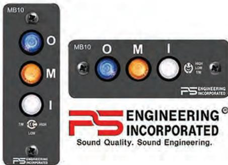
MB 10-is a 3-light 75 MHz Marker Beacon receiver and indicator. This provides the necessary Marker Beacon lights and audio indications necessary for an Instrument Landing System (ILS) approach. A switch labeled Hi/Lo/TST allows the pilot select high or low sensitivity as well as test and mute modes. • Height: .95 inches • Width: 2.80 inches • Depth: 4.85 inches • Warranty: 1 year • Unit is TSO'D
