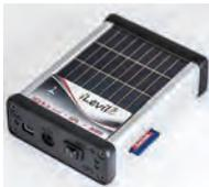
The next generation of iLevel is here! and it brings exciting features and capabilities. This portable tool combines the latest in GPS, AHRS, ADS-B, and Data Recording technology to bring pilots an affordable backup solution that is both Android and iOS compatible. The internal GPS and AHRS provides all the navigation information you need to turn your tablet into a real glass panel. The embedded dual band ADS-B receiver allows you
