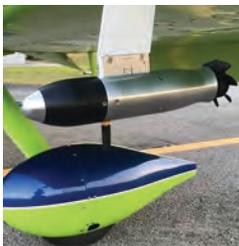
The BOM (Broadcasting Outer Module) is the first and only aerodynamic pod that mounts under the wing of the aircraft. All components are incorporated into the BOM, making it a fully independent, completely wireless, self-powered, all in one avionics device. Avionics include WAAS GPS, ADSB-in, AOA, Air Data (Altitude, Airspeed), AHRS (Attitude, Directional Gyro, Turn Coordination, rate of turn, VSI) and outside air temperature. Once it is installed, the BOM connect via Wi-Fi to a tablet inside
