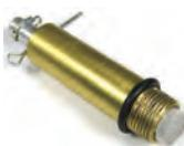
This Bendix Mag Lock works on S4 and S6 and other Bendix Mags. To use simply place a cotter pin loosely into lower plunger hole. Screw sleeve into magneto case. Align red slot in plunger parallel to mag tooth gear. Remove cotter pin to engage gear tooth. Dimension: 2-3/4" x 1/2" x 3/4"
