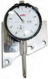
The Valve Wobble Test Fixture for parallel valve Lycoming engines is used to comply with Lycoming SB-388a. Quality made of aluminum and alloy steel, it is easy to use with no set screws or feeler gauges required. Allows direct reading of wobble from dial indicator. Note: Will work on a angle valve engine.
