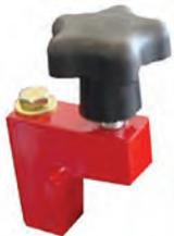
These simply bolt to the head and the knurled knob screws down to compress the valve spring allowing the shaft to be slid out with no spring pressure.
