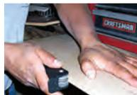
The core recessor is a new product with the purpose of serving as an efficient tool that makes the process of removing core cells in Nordam Panels and composite fiberglass more efficiently. Thus, it reduces time for edge fillers, which are necessary procedures to customize aircraft cabinets, floorboard, vanity's headliners, valance panels, etc. Is light weight, easy and safe to use. Core panels from 1/8 to 3/4 inch with no adjusting. Requires no electricity.
