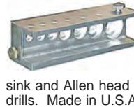
This tool provides a fast, simple way to drill bolt heads with virtually no broken drill bits. The tool is made of 6061T6 hard anodized aluminum for durability. Fits 3/16" to 5/8" dia. bolts and works on hex head bolts, header bolts, 12 point countersink and Allen head cap screws. Includes drill bushings and two cobalt drills. Made in U.S.A. .... P/N 12-16600 ..... **\$71.75**
