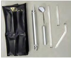
Kit consists of aluminum 2-cell holder, 1-cell holder for use in small areas, 6" straight Lucite conductor, 4" curved Lucite conductor for lighting around corners, 2-1/2" straight conductor for pin-point lighting, and clip on mirror which attaches to any of the Lucite conductors. When used with curved conductor it can virtually make light available around a corner in a full 360° arc. Operates on penlight batteries (not included).....P/N 12-14900.....**\$19.95**
