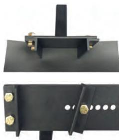
Adjustable jack pad with rubber protective strip for spring steel landing gear. (fixed-gear Cessna 150, 172, 182, etc). Just tuck the pad underneath a landing gear leg and bring a floor jack up to it, efficiently lifting the wheel for tire/hub work.
