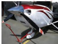
The "QUICK-FOLD COMPACT TOWBAR" also known as the "QFC--Towbar™". No more back breaking, bend over towing. Simply attach the QFC-Towbar™ extension to your already existent Cessna tow bar and stand up straight. An added extension of 33". Folds flat and is stowed securely along side the factory tow bar.
