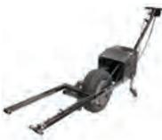
**Features:** • No Flammable gasoline needed in hangar • Easy To Use • Infinite Speed Control • Versatile Applications • Push button forward and reverse controls • Nose gear quick attach for easy nose gear hook up. • The adjustable fork height fits virtually any light aircraft • Trickle charger for battery • Large 16 x 6.50 - 8 turf tire • For aircraft weight of 3500 to 4500lbs. Battery not included.. P/N 13-04513 ..... **\$1,534.00**
