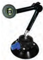
This one mount can operate as a compact suction cup, allowing a close position to the glass of 3.25 inches. It can also operate as a standard suction cup mount extending to 10.5 inches. The Mount utilizes one vacuum suction cup with a built-in finger pump that informs you if the mount is losing suction. Give it a couple pumps and it is quickly back to full strength. **Note:** You must have a device holder to use this mount.....P/N 13-19509 .....\$194.00
