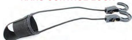
RANS has developed a control lock that attaches to most models. The lock consists of a bungee cord, a couple of hooks and cap that slips over the top of the control stick. Allows for bungee tension to be set for a particular model. Not hard bolted so if an outside force against the control surfaces occur, the bungees will absorb the load.
