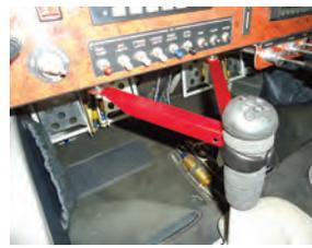
These control lock is easy to install and positively locks the ailerons and elevator of the aircraft models listed below. Gust lock is manufactured using 6061T3 aluminum. The control stick clamping portion has a protective sleeve to prevent damage to special control handles. The latching mechanism is tow locking buttons that cannot come loose until released by the pilot which insures the owners that
