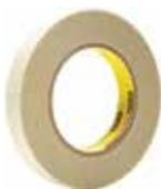
Constructed with a woven fiberglass backing, 3M™ Glass Cloth Tape 361 features a pressure sensitive silicone adhesive for applications requiring high-temperature resistance, high adhesion and clean removal. It is often used for high temperature applications such as sealing ducts and as a back-up strip for submerged arc welding.
