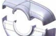
This Cessna 150 Cowl Nose Cap (shaded part shown in cowl assembly figure), Upper Cowl is a replacement part within the upper cowl assembly. This part is a NEW part not a USED or refurbished part and replaces Cessna part number 0452002-6 and 0452011-2. This part is fiberglass and comes without paint. This part fits aircraft with the 150 HP STC SA4795SW or equivalent conversion.
