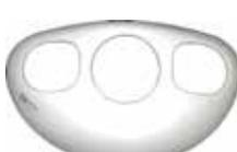
Same shape and size as used on the Piper PA-14. Can be used on the same aircraft as listed for the MC-3A design. For builders not wishing to use an electrical system and is seen on most Pitts Specials built for competitive aerobatics. 35" wide x 21" high. Center opening 9-1/4" dia .....P/N 05-01184 .....\$153.00
