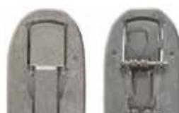
The H-5000-2 style latch is a unique spring-loaded, trigger action latch for cowl and access doors. Made of corrosion resistant steel. Rivet or spot weld to structure. Bolt Offset: .132. Trigger Offset: .102. Max. Depth: 1.23
