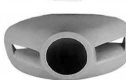
This nose cowl was designed for the T-18 pressure cowl system. A 4-inch prop extension is required and it is generally used with the MC-5 Bottom Cowl. Measures 36" wide by 20" high. Face of center opening 12-5/8" O.D. P/N 05-00551 .....\$157.80
