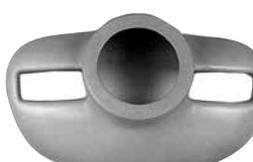
Originally made for the Thorp T-18, this cowl has been used on several other types. The starter ring is enclosed when used with the Lycoming. Makes a nice front end on the CA-61 & CA-65. Measures 35"W by 19.5" high. Face of center opening 13-1/2" O.D. P/N 05-01176 .....\$151.80
