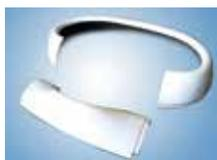
Styled after the Piper Comanche, this cowl can be used on just about any homebuilt powered by the Lycoming engine. It is made in two parts, allowing the easy removal of the cowl without having to remove the prop. Used on the following airplanes: Starduster I and II, Playboy, EAA BiPe, Jodel D-11, Tailwind, Tempete & the Skybolt. Measures 35" wide by 21" high. Will accommodate a spinner approx. 12" in dia. P/N 05-01180 .....\$123.85
