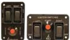
The EA-15000 is an approved ignition switch panel to control two magnetos and a starter in a conventional ignition configuration (magneto to magneto). The panel comes in two versions, a horizontal one and a vertical one. This set of ignition switches is approved to replace the outdated and venerable rotary key-switch.
