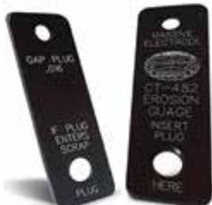
Champion CT-482 spark plug erosion gauge provides an easy, accurate method of determining whether your plugs have reached their maximum wear limit. Calibrated to reject plugs after their electrodes have eroded to at least one-half their original thickness.
