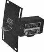
Warns by light and horn of any danger of an approaching stall regardless of the flight maneuver. Never signals unless a stall is imminent. Consists of an instrument panel unit (fits standard 2.25" hole) containing a warning horn & signal light, and a small vane wing unit which operates a relay. Operation of the instrument doesn't depend upon air speed but rather on the air flow conditions of the wing. Complete with installation kit & instructions. Installation time: 2-6 hours.
