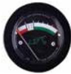
Lift Monitor is FAA approved for installation on all GA aircraft, not just experimentals. The low cost of the Lift Monitor and simplicity of installation leave little excuse for not availing yourself of the safety and performance afforded by an AOA system. Working completely independently of all other aircraft systems, installation requires only a log book entry on the part of your mechanic.
