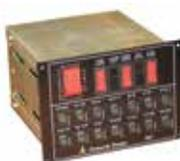
The Radio Stack Power Panel is designed to fit neatly in the 6.25" radio stack format. It is well suited for LSA and light aircraft applications, offering a new degree of flexibility in modern "Glass Panel" equipped aircraft. The power bus is split into three segments including the Main Bus, Radio Bus and the Essential Bus. The Radio Bus is switched and filtered. The Essential Bus can be
